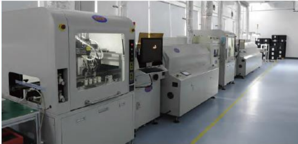
Auto Conformal Coating Line
